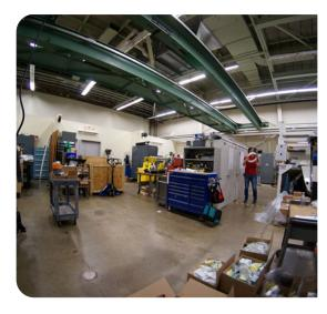
The DEVCOM Armaments Center's Autoloader Lab is a 2500 sq ft facility capable of housing, integrating and bench testing a variety of autoloader systems.
