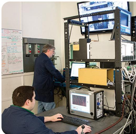
*The Breech Fatigue Simulation Facility is a dedicated Department of the Army facility established to provide cost effective, safe fatigue life determinations of all large caliber armament breech assemblies through dynamic hydraulic medium pressure cycling.*
