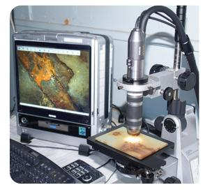
The Corrosion Testing Facility (CTF) is a dedicated Department of Defense facility established to provide an inhouse and cost effective means to investigate, experiment and evaluate the corrosion resistance of Army materiel.
