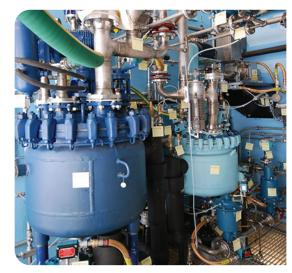
The Flexible Nitration and Crystallization Pilot Plant is a remotely operated chemical synthesis and crystallization facility designed to scale-up energetic and related materials to bridge the gap between lab-scale and full-scale production.
