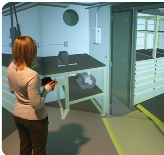
*The Immersive Engineering Laboratory (IEL) is a system of 3-dimensional (3D) technologies designed to enhance engineering reviews by immersing users in a 3D Computer Aided Design (CAD) model.*
