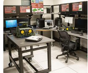
The Joint Precision Airdrop System (JPADS) Software Engineering Laboratory (SEL) is used to verify and validate contractor software deliverables using Hardware-in-the-Loop simulations.
