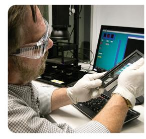
The Optical Surface Quality Standards Laboratory, certifies the Surface Quality Standards also known as Scratch and Dig, for the Manufacture, Assembly & Inspection of Optical Components for Fire Control Instruments.
