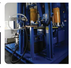
The R&D-Scale Explosives, Mixing, Pressing and Loading facility produces and post-processes explosive formulations to complete explosive characterization testing. The facility can fabricate explosive tablets, pellets and billets of diverse composition for formulation development and munition prototyping.
