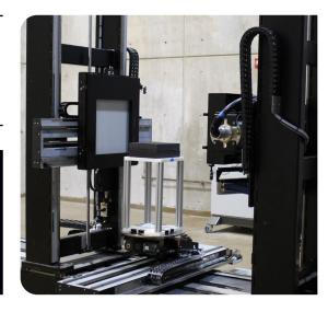
The DEVCOM AC Radiographic Laboratory is primarily used for nondestructive imaging and analysis of items. These items may be energetic in nature, require quality control, need examination prior to and after destructive testing, or are of an unknown configuration.
