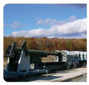
The Soft Catch (SCat) Gun Facility validates structural models and designs without the logistics and cost of extensive live fire testing.
