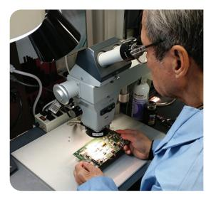
The Soldering Technology Laboratory (STL) is a dedicated Quality Engineering & System Assurance (QESA) facility established to provide inspection of the soldered connections of circuit boards and components for the Telemetry hardware and other DEVCOM weapon systems.
