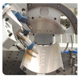
Benét's Stress Analysis Laboratory specializes in the measurement of residual stress and retained austenite using X-ray diffraction. These measurements are often critical in verifying various manufacturing processes such as autofrettage, cold working, and heat treatment.
