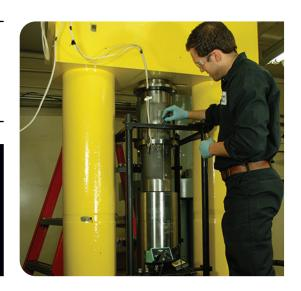
Benét Laboratories' Tube Fatigue Laboratory provides a unique capability to facilitate constant amplitude cyclic hydraulic fatigue testing on cannon and artillery to establish their Safe Service Lives.
