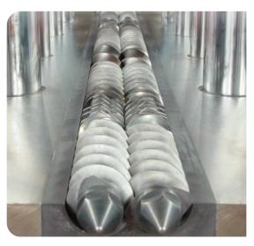
The 40-mm Twin-Screw Mixer/ Extruder (TSE) Facility is a continuous remotely operated, flexible facility that can significantly enhance safety and environmental considerations during the processing of energetic materials.
